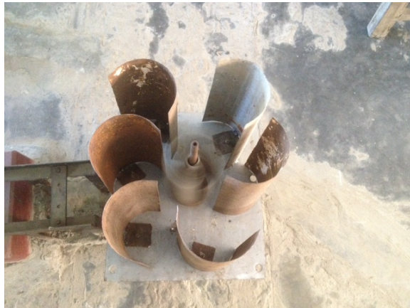
Fig. 2: Experimental set up of savonius rotor with six deflector blades
